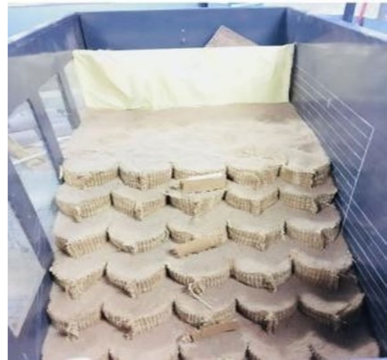
Figure 3.2 Coir geocell retaining wall [13]
